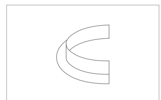
No. 8034/1 Pillar connection semi-circle Ø 250 – 500 mm in increments of 50; height: 20 mm, width: 20 mm, thickness: 1.5 mm Important: max. tolerance pillar diameter \pm 3 mm; adaptation required.
